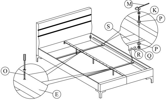
Step 6: Tighten all the 4 corner ,follow by assembly of the slat holders with LVL slats as shown.
